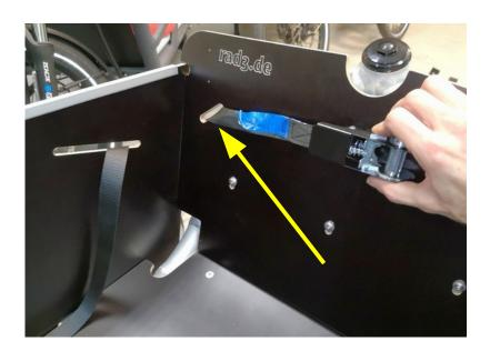
Fig. 11-1: Thread the tensioning strap, in front and to the left
