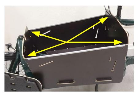
Fig. 8: Insert side parts, tighten nuts with torque
