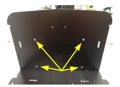
Fig. 4-1: Put on rear wall, screws 25 mm K-washers Cap nuts
