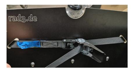
Fig. 11-3: Tighten with ratchet
