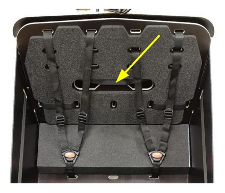
Fig. 11-2: IMPORTANT for safety! Thread the belt, Include seat back
