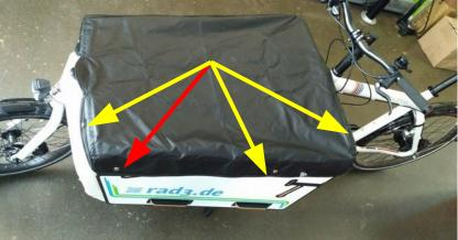
Fig. 13-3: Pull the tarpaulin tight, press studs on the right are mirror image
