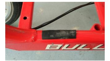
Fig. 1-1: Protective supplement Paint protection, noise reduction
