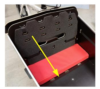
Fig. 12: Insert cushion (shown without straps)
