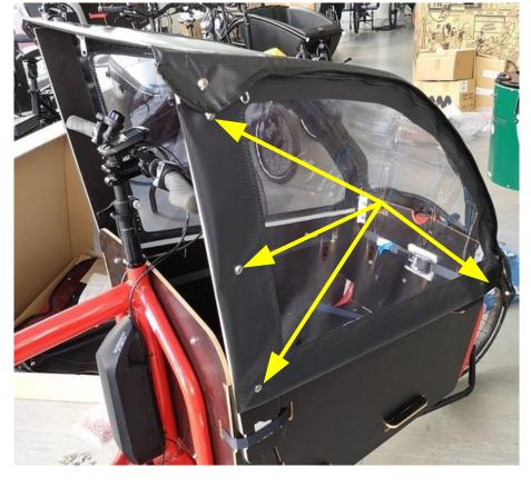
Fig. 14-8: Pull the sides into shape, set more press studs
