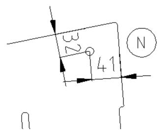
Fig. 14-12x: 32 mm from wooden edge (approx. 34 mm from profile edge)
