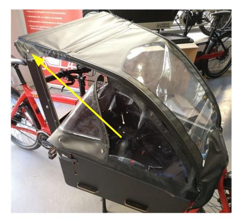
Fig. 14-7: Pull handlebars up and shape, set first push button
