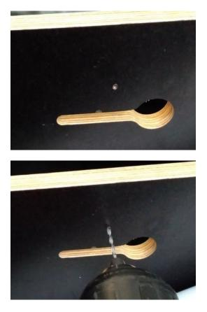
Fig. 13-5: Pre-piercing and pre-drilling
