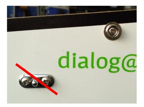
Fig. 13-7: Tenax screwed on (photo old model)
